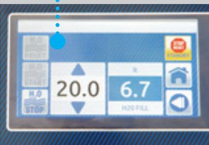
Provided with an automatic litre counter for pre-setting of the litres of water to be poured into the tank. Useful in case of even partial milk reconstitution.
